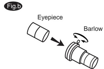
In addition to increasing magnification, the benefits of using a Barlow lens include improved eye relief, and reduced spherical aberration in the eyepiece. For this reason, a Barlow plus a lens often outperform a single lens producing the same magnification. However, its greatest value may be that a Barlow can potentially double the number of eyepiece in your collection.
